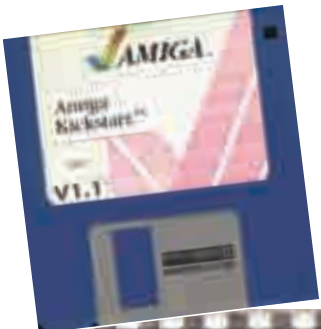
» Below: The original Kickstart came on floppy disk but by the time of the A500 it was a ROM chip on the Amiga motherboard.
